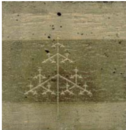
Antenna on Concrete With Polymer overcoat
